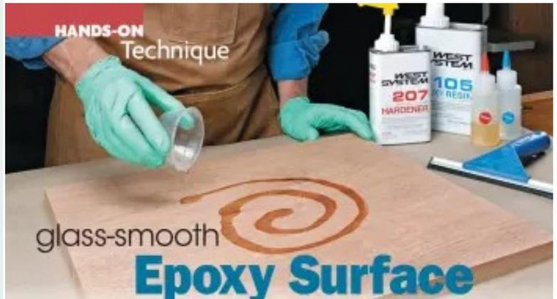
Versatile epoxy fills pores and creates a smooth, durable moisture barrier for a fine furniture finish.
