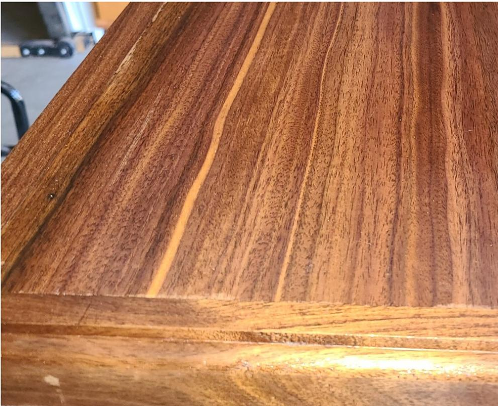
And here is walnut surface after a thin coat of sanding sealer, light sanding with 320 grit, then 3 coats of glass poly thinned 50% with paint thinner. Each poly coat was wiped on with lightly saturated rag then wiped off as much as possible with the same rag. I allowed 3 hours dry time between each poly coat but 2 hours would have also been ok. Dries to touch in only a few minutes so dust isn't a problem. No sanding at all between coats, only light sanding of initial sanding sealer.
