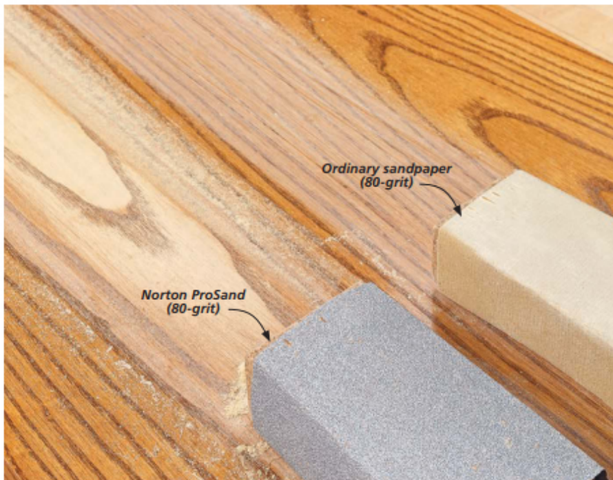
▲ After 50 strokes with both premium and ordinary sandpapers, you can see the difference in the amount of material that is removed. The higher-quality abrasives in the premium sandpaper stay sharp longer. This means they cut faster and don't break down as quickly.
