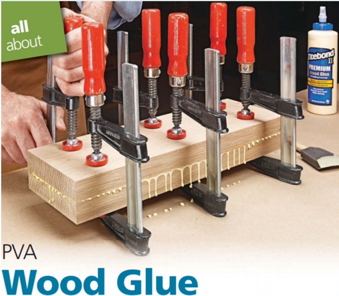
How PVA Wood Glue Works The polyvinyl alcohol surrounding the resin particles chemically bonds to the cellulose in the wood. The PVA resin contributes to a strong glue bond.
