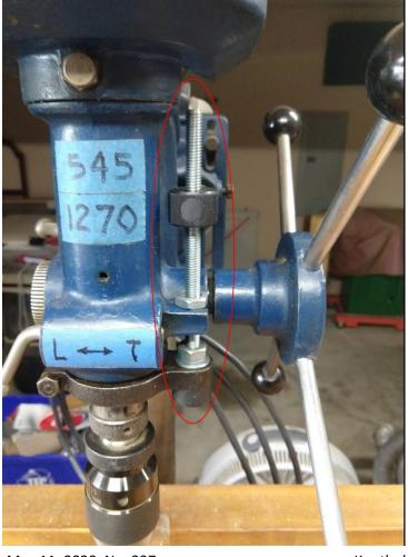
I could not be happier with the upgrade to my recently acquired 1940's vintage drill press. I replaced the traditional, double-nut, depth stop, which took "forever" to screw up and down, with a push-button, slide-adjust nut.
