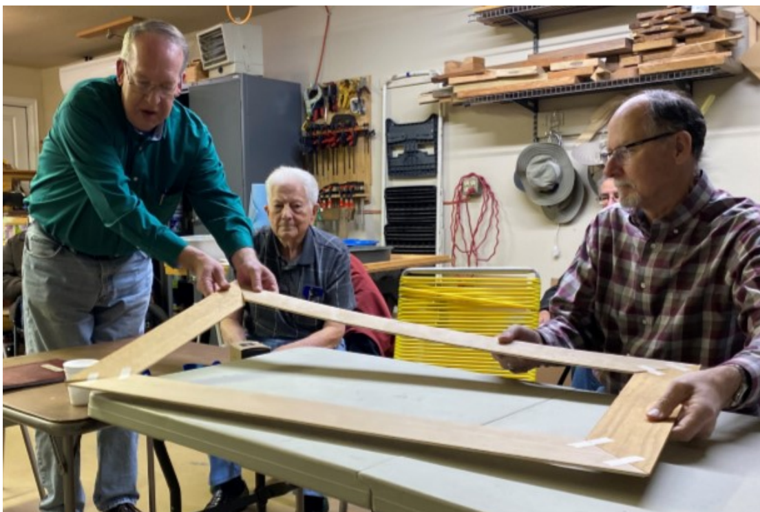
Mike cut this picture frame on his table saw using the gray, 45 degree sled shown above; all 4 joints fit together perfectly with no gaps in the joints
