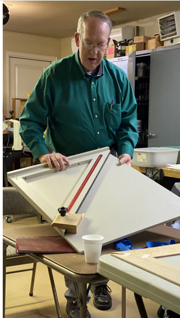
Mike Ruttgen shows us his triangles for cutting precision 45 degree crosscuts
