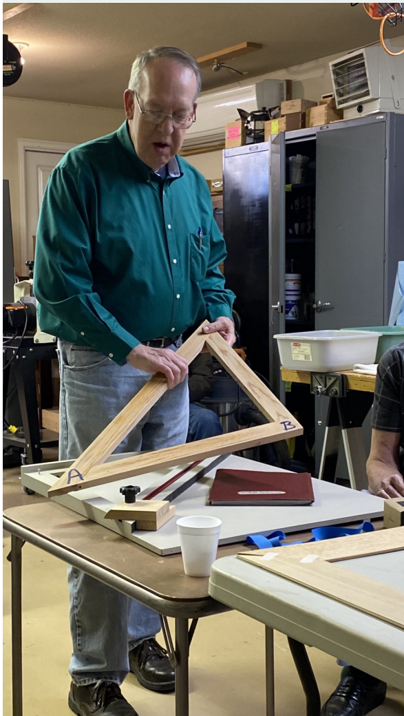
Mike Ruttgen shows us his triangles for cutting precision 45 degree crosscuts
