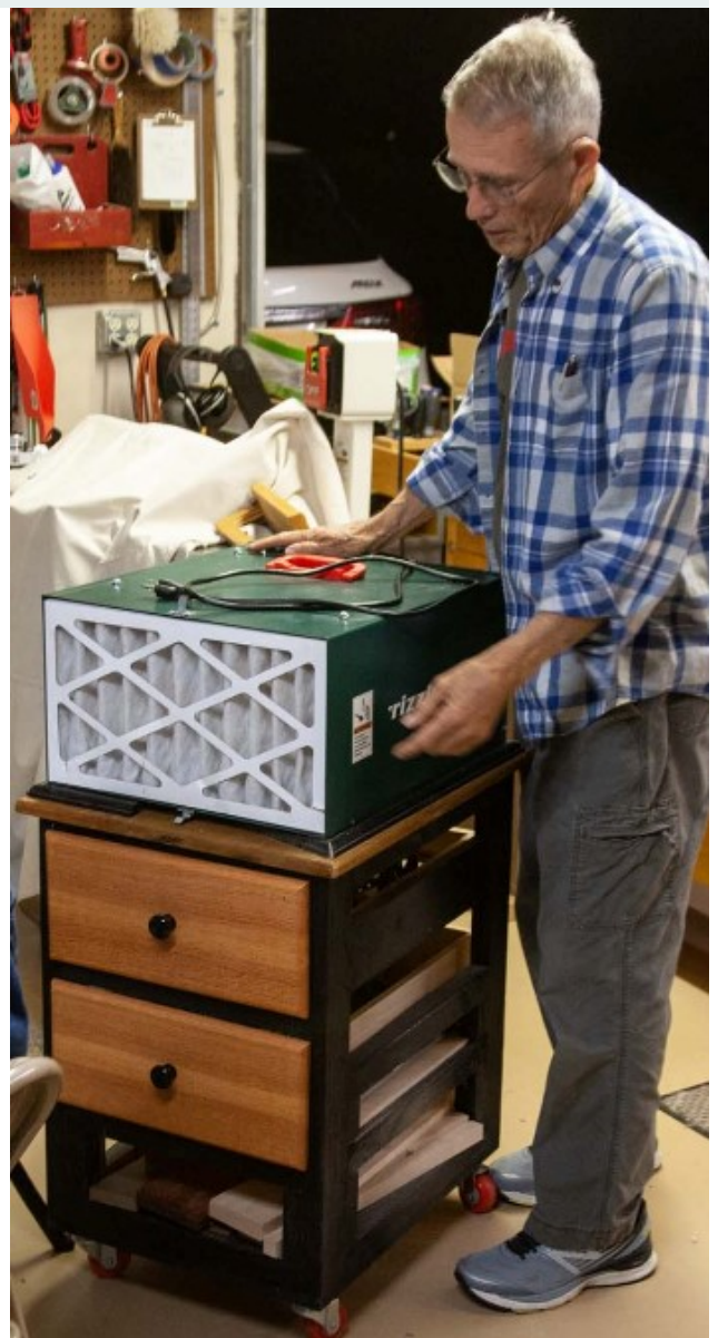
Earle mounted his Grizzly hanging air filter unit on a rolling base so that he can easily relocate the unit near the dust source.
