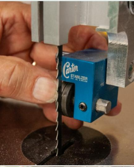
Masking tape is just the right thickness, when added to the blade, to property adjust the upper and lower blade guides.
