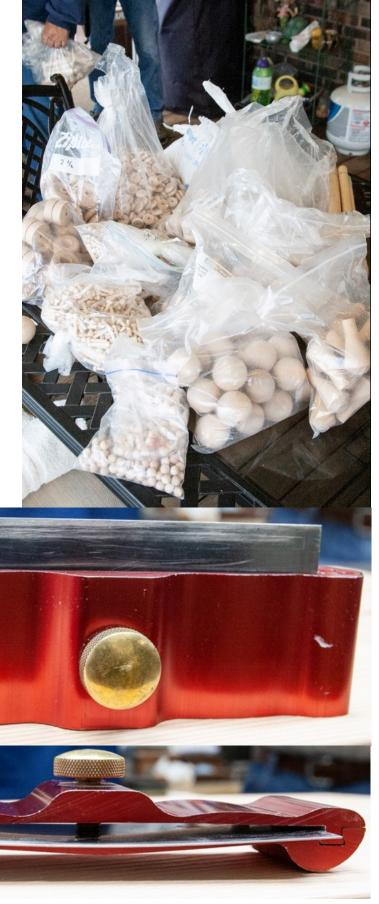
Front and side view of a card scraper holder. Note how the knurled bolt secures the blade against the curved side.
