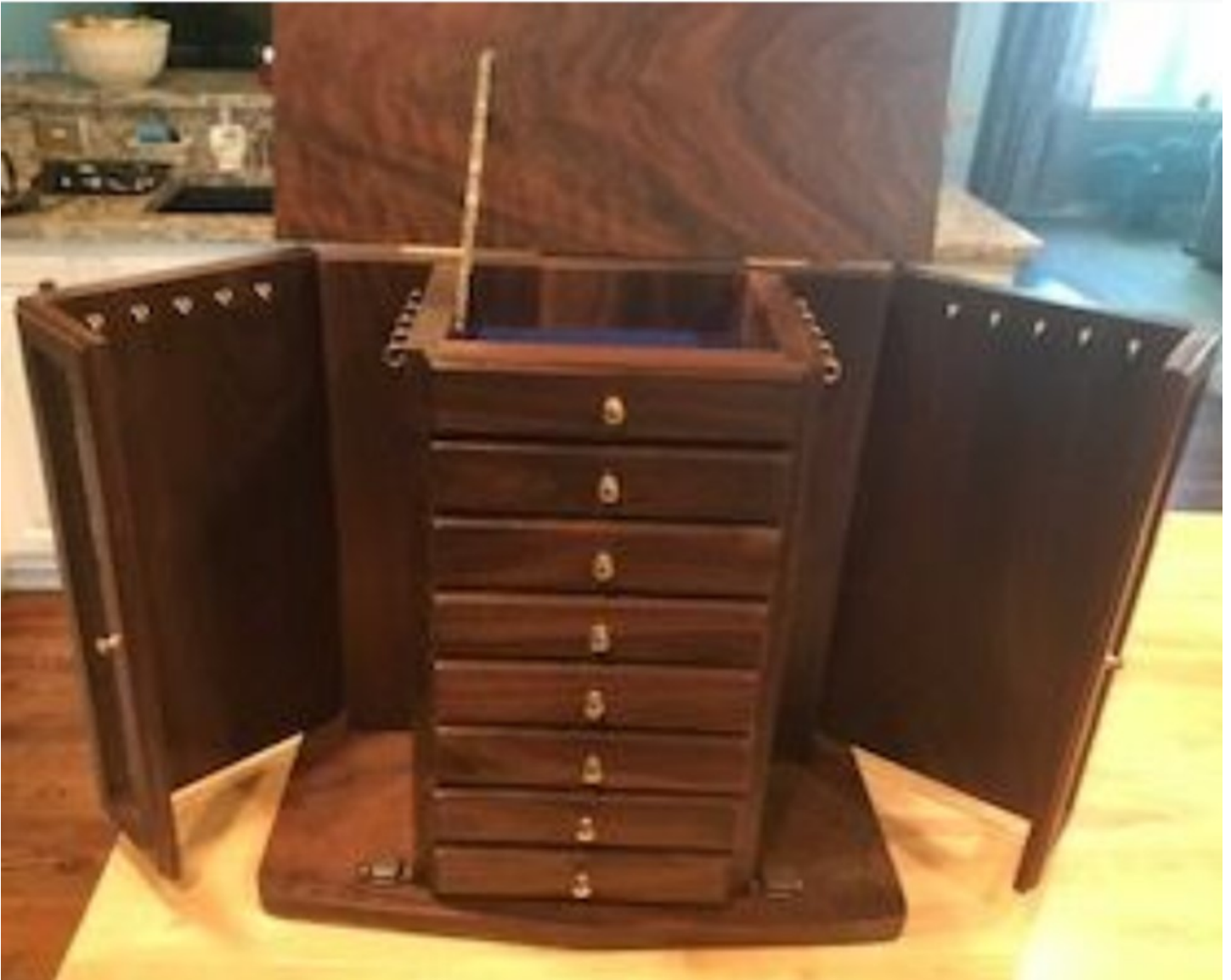
A classic heirloom jewelry box made by Vinton Knarr for his granddaughter. The wood is walnut finished with a base coat of Danish Oil a couple of top coats of Minwax Wipe-on-Poly.
