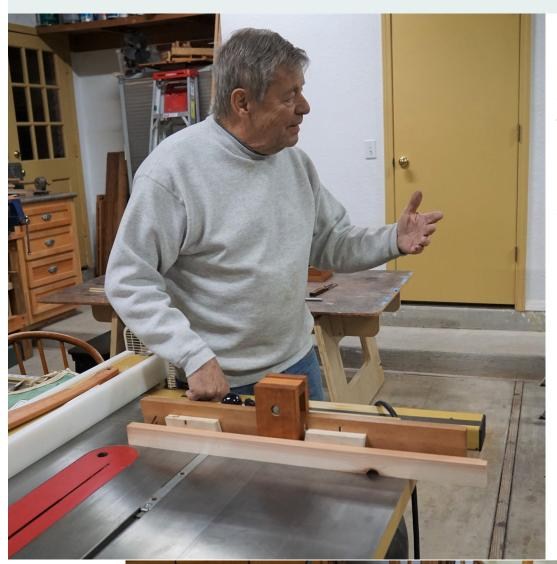
Robert showed how he souped-up his Incra miter gauge used on his Powermatic table saw. He added a wood facing with a stop block and attached a second facing to preserve the setting of the stop block.
