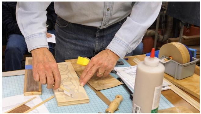
Pictured is Bill spreading a uniform layer of glue to the substrate. Note the roll of tape in the background. It is used to seal the veneer along adjoining edges to prevent creep. Also, several types of glue can be used such as Titebond, hide glue and glue made especially for veneers. His recommendation is Unibond One that is sold on the Internet.
